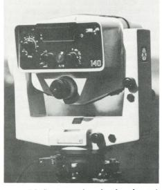
AGA Geotronics has developed a unique angle measuring system for their brand new total Station Geodimeter (140). The new system makes it possible to measure the exact angle in a single face measurement, as opposed to the conventional way in a two face measurement,
